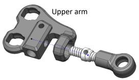
Screw the turnbuckle to the upper arm. (Normal thread side)
